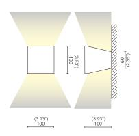
Characterized by the symmetrical cuts, Mia is a dou-ble emission wall lamp made from epoxy polyester powder coated aluminium and it is equipped with Chip On Board technology high efficiency LED light sources and driver. Its degree of protection against the penetration of dust, solid objects and liquids is IP20.
