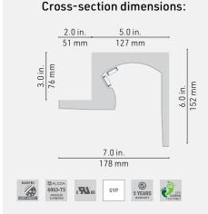
The **NIDUS** profile is an easy and affordable solution for lightgrazing a wall, while keeping the **LED source concealed** and the **corner visually intact**. Install over 2×3in. beams/joists, without the need to build elaborate wood structures, level with the gypsum panels, then mount the LED profile(s) at the position yielding the desired beam direction. Great above blinds or curtains!
